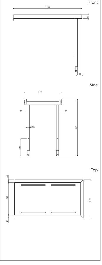
Handling System for Rack Type Dishwasher Loading&Unloading Table, 1100mm
